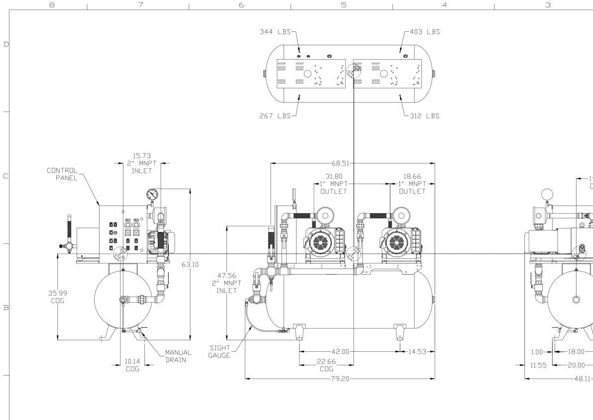
NDTE: A MINIMUM DF 24" CLEARANCE IS RECOMMENDED AROUND THE ENTIRE UNIT. 8 7 6 5 4 3
