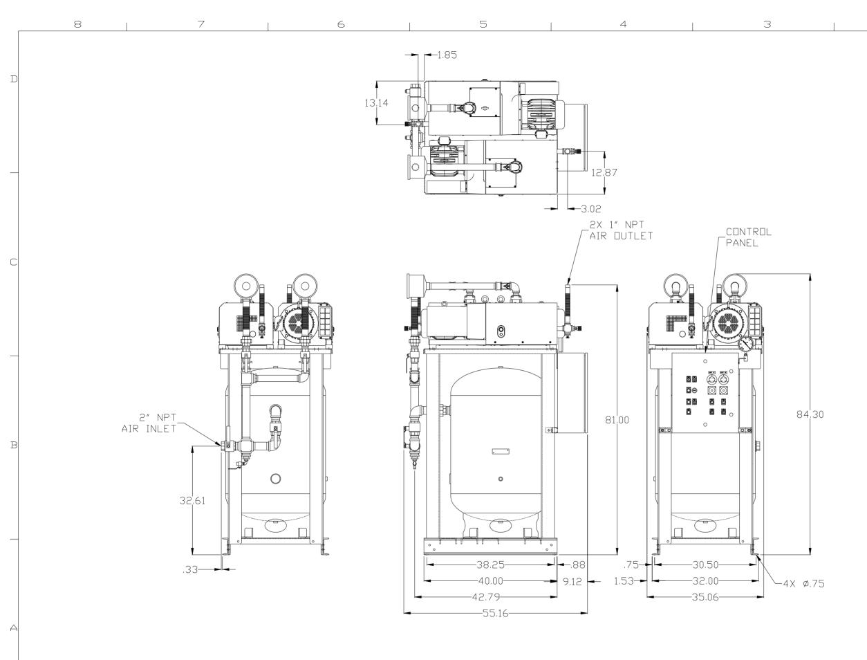
NDTE: A MINIMUM DF 24" CLEARANCE IS Recommended around the entire unit.
