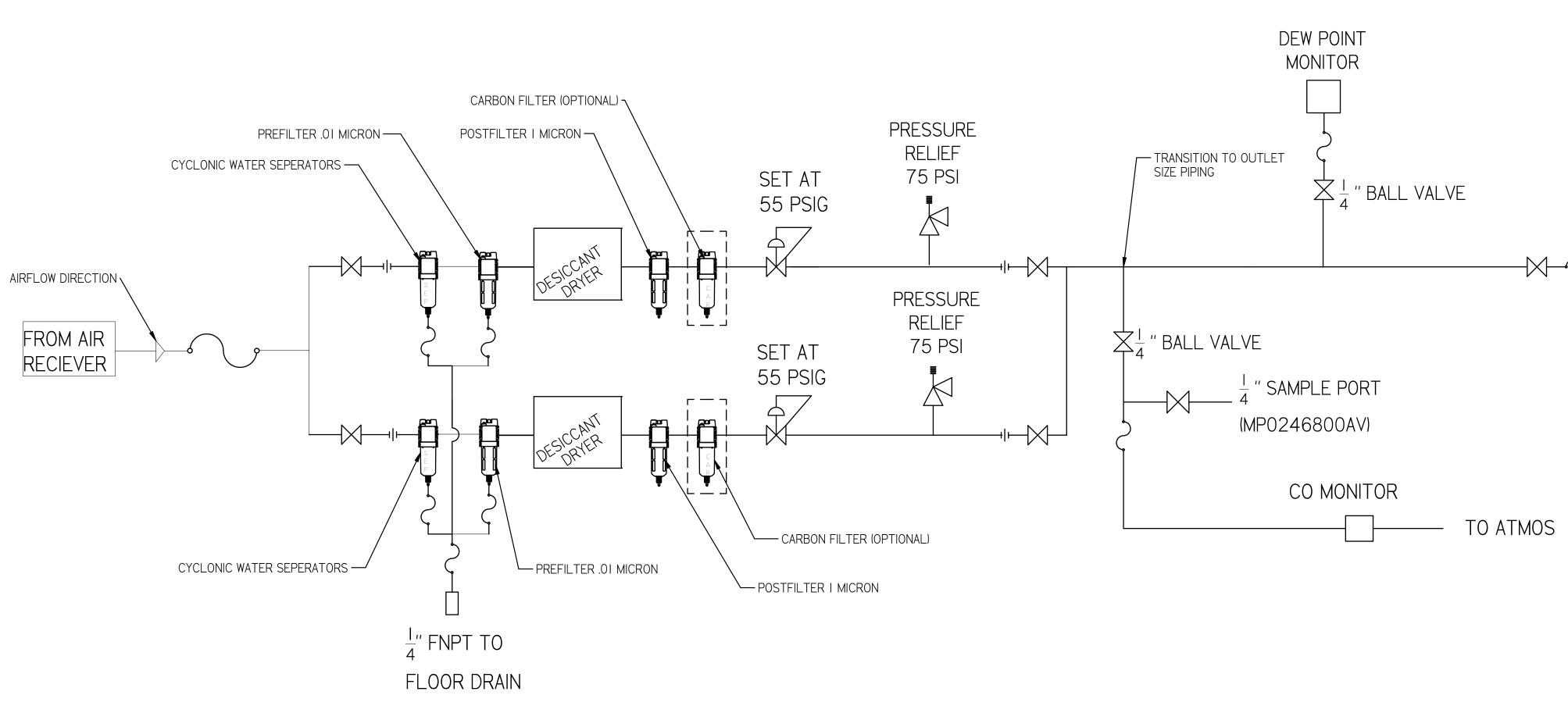
MSQI5A6 MEDICAL OPEN SCROLL 15 HP QUADPLEX WITH 240 GALLON TANK MEDICAL DRYER FLOW DIAGRAM
