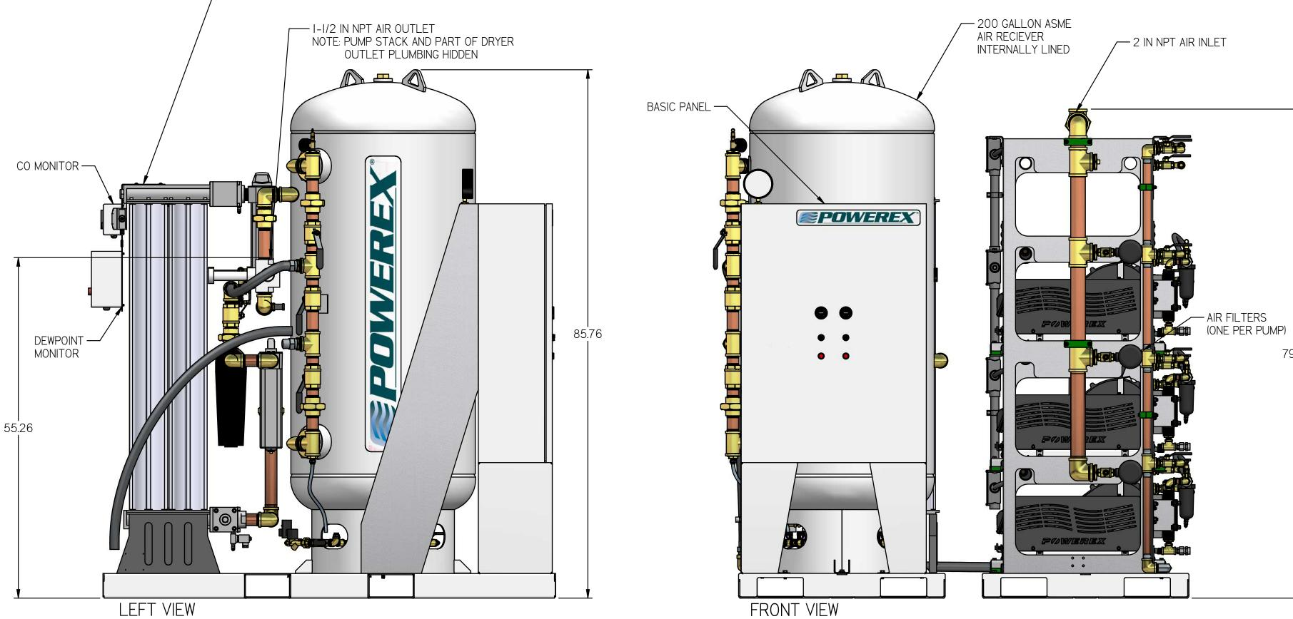
— 2X DESICCANT DRYER WITH DEWPOINT MONITOR, CARBON MONOXIDE MONITOR, PREFILTER, AFTER FILTER, & OPTIONAL CHARCOAL FILTER
