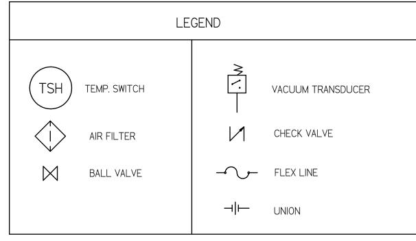
NOTES: I) TSH - TEMPERATURE SWITCH HIGH 2) PER NFPA THE SYSTEM WILL REQUIRE A SOURCE VALVE (SUPPLIED BY OTHERS). 3) OUTLET SILENCER AND FLEX HOSES SHIP LOOSE FOR FIELD INSTALLATION.
