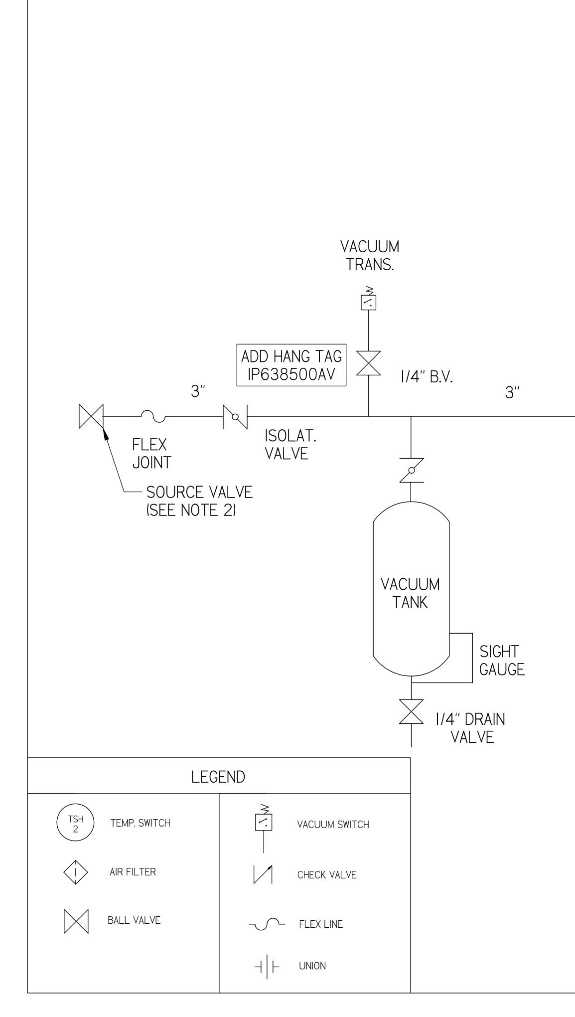
NOTES: I) TSH – TEMPERATURE SWITCH HIGH 2) PER NFPA THE SYSTEM WILL REQUIRE A SOURCE VALVE (SUPPLIED BY OTHERS)
