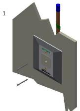
Remove the mounting screw from the existing front body.
