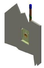
Clean any loose chips and debris from the back body outlet.
