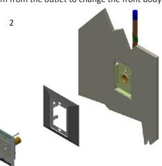
Remove front outlet assembly and trim plate.
