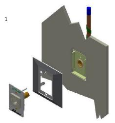
Place the original trim plate on the wall and install the front outlet conversion body into the back body.
