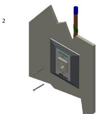
Once the components are placed into the back body, install the new mounting screws.
