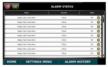
The Alarm Status screen shows a list of all possible alarm conditions for the maximum number of gases and input signals available in the Powerex FirstCall™
