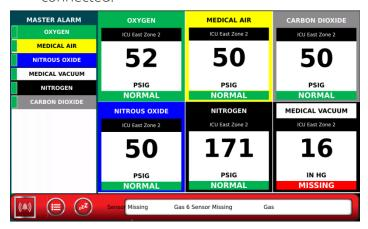
2. Mismatch – panel detects a transducer connected, but it is the wrong gas type.
