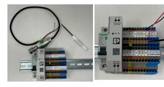
It is important that the sensors are wired to the correct terminal block. Per NFPA 99, an alarm will sound for cross-connected sensors.
