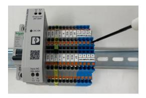
Install the sensor wires into the appropriate terminal block. There are enough terminal blocks for up to 8
