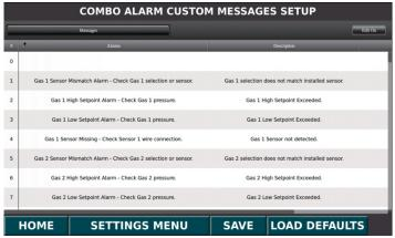
The Powerex FirstCall™ Alarm System allows the user to program specific instructions for each alarm event.
