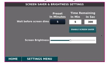
The Powerex FirstCall™ Alarm System is factory-set with a 5 minute screen saver. The screen saver dims the panel to 10% after 5 minutes. This time limit can
