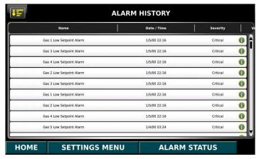
The Alarm History screen shows a record of all alarm events up to 32, including the specific alarm condition and the date and time of the alarm event.
