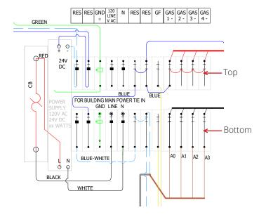
The image below shows a sample terminal block layout from the alarm panel with the top and bottom circuits labeled and correspond with the labeled circuits on the sample wiring diagram above.
