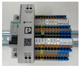
Ground wire – Strip ½" of insulation and connect the ground wire to the appropriate terminal block (GND).
