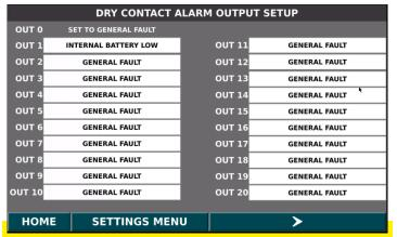
Standard dry contact output is on terminal block "O0" for General Fault. 20 adjustable outputs are available standard. Adjustable outputs must be wired directly into the terminal strip on the PLC.
