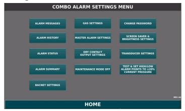
The Area Alarm settings screen will not have a button for "Master Alarm Settings."
